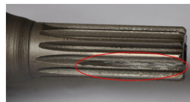
Fig. 9 The implanted fault on the sun gear
