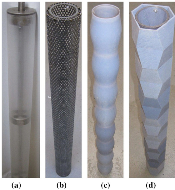
Fig. 23 Tested models, a circular cylinder, b shrouded cylinder, c wavy cylinder, d faceted cylinder [182]
