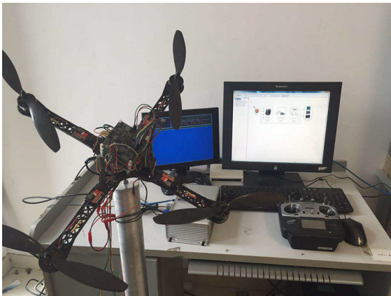
Fig. 2 Hardware-in-loop-simulation quadrotor testbed
