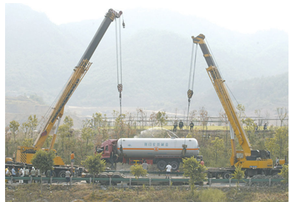
Fig. 2 Dual automobile cranes system
