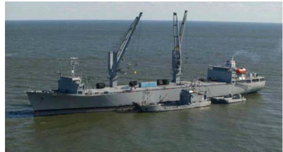
Fig. 1 Dual shipboard cranes system
