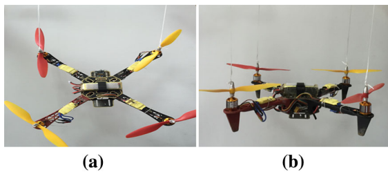
Fig. 4 Measurement method of rotational inertia. a Two-line method. b Four-line method
