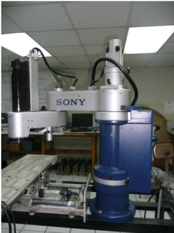
Fig. 4 SCARA robot. The first link corresponds to system \Sigma_4
