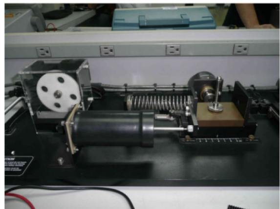
Fig. 2 Mass–spring–damper system that corresponds to systems \Sigma_1 and \Sigma_2
