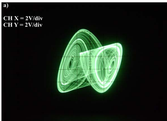
Fig. 6 Experimental projections of double-scroll attractor of the analogous Chua's circuit: a (y) \times (x) and b plane (z) \times (x)
