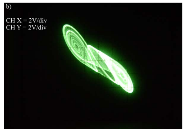
Fig. 6 Experimental projections of double-scroll attractor of the analogous Chua's circuit: a (y) \times (x) and b plane (z) \times (x)
