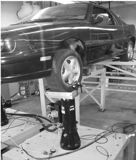
Fig. 3 Full-vehicle shaker test setup
