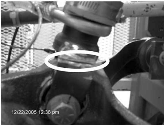
Fig. 21 Complete cut in shock clevis
