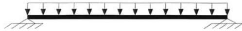
Figure 1. Schematic diagram of a pinned-pinned planar rod. The dynamics is computed by the method of finite elements.
