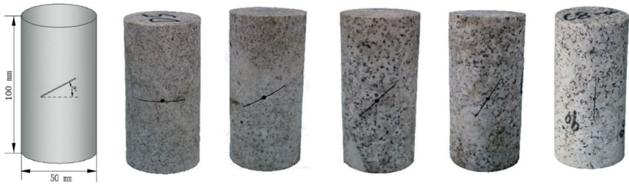
Fig. 2 Granite sample with pre-existing cracks
