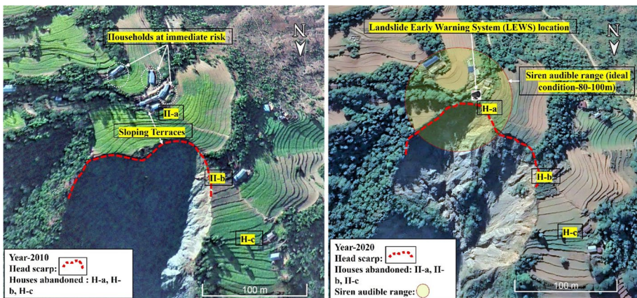
Fig. 2 Methum landslide head scarp region: Household at risk and sloping terraced farms in the crown area (left photo 2010) which has already collapsed in the right photo (2020) with the LEWS station; siren audible range, and H-a, H-b, and H-c represent three abandoned houses
