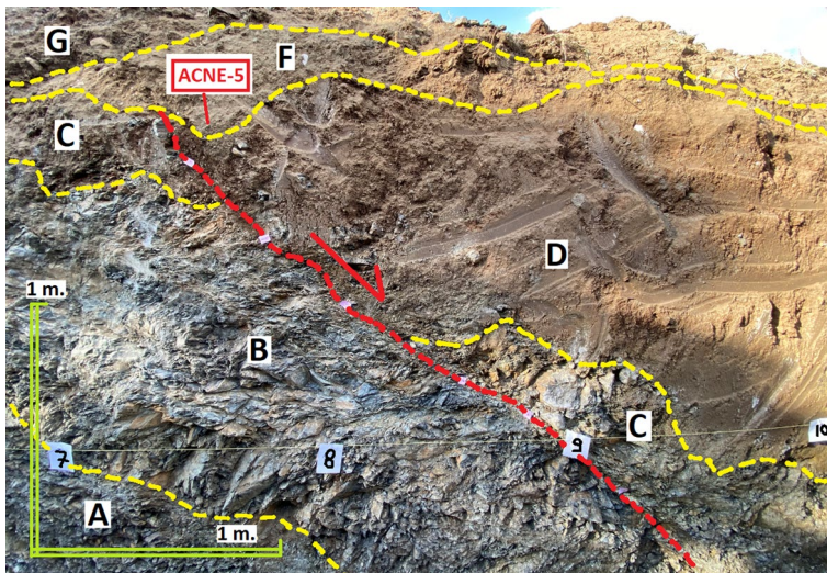
Fig. 14 Detailed view of the cross section between 7th and 10th m from SW to NE in Trench-3 (fault lines in red, unit boundaries in yellow) (explanations of units and faults are in text) (see Fig. 13)
