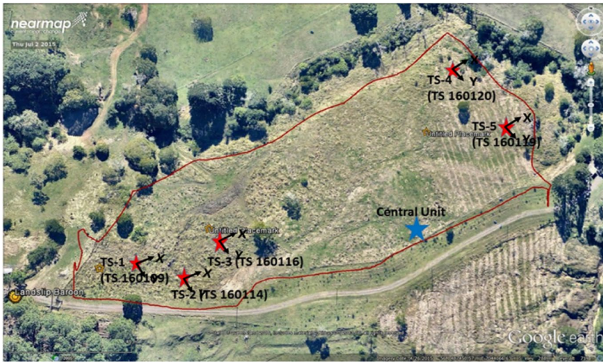
(a) Sensor locations at the slope in Queensland, Australia (X denotes downslope direction)
