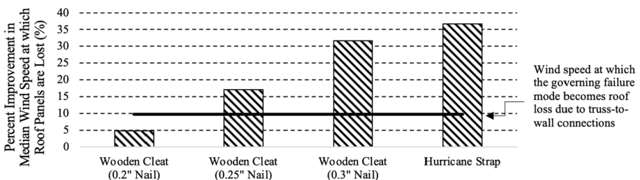
Fig. 5 Changes to median wind speed at which roof covering is lost due to modifications at the purlin-to-truss connection. Note: Percent improvement from the previous case at 92 mph (Base structure: nailed purlin-to-truss connections)
