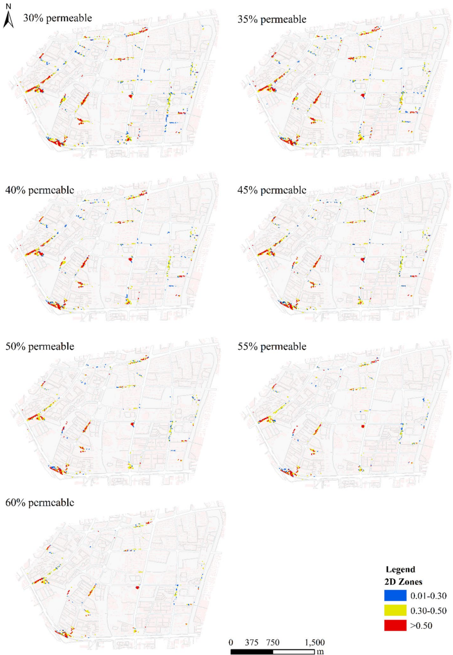
Fig. 9 Flood risks for 30–60% permeable surfaces
