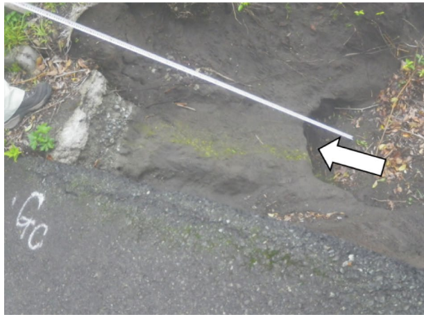
(b) Nearby head scarp and piping hole
