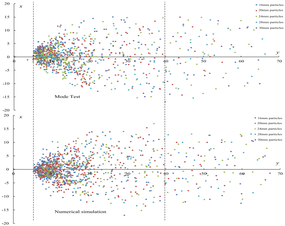
Fig. 23 Accumulation and distribution of particles with different sizes in tests and numerical simulations
