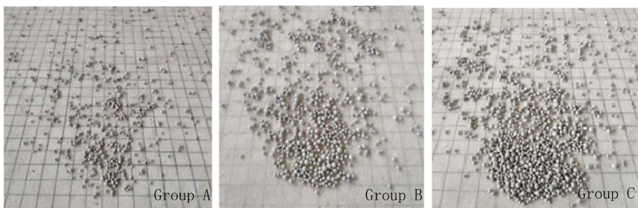
Fig. 10 Particle distribution at end of accumulation body in Groups A, B and C
