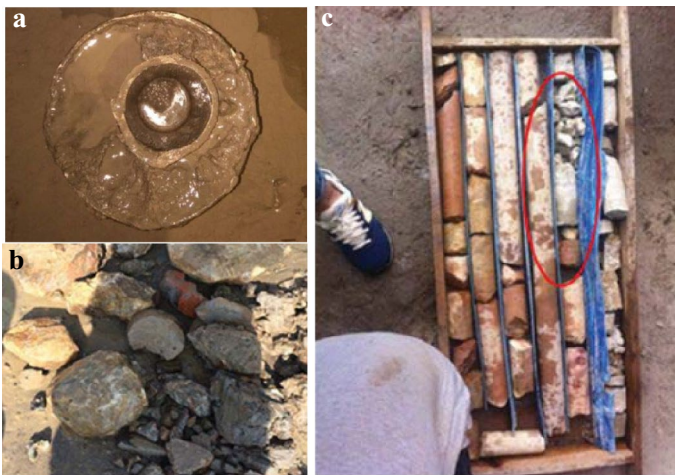
Fig. 16 Photographs of in situ slurry grouting. a , b and c are sealed grouting hole, cement slurry solid and drill core after grouting (Gao 2017)
