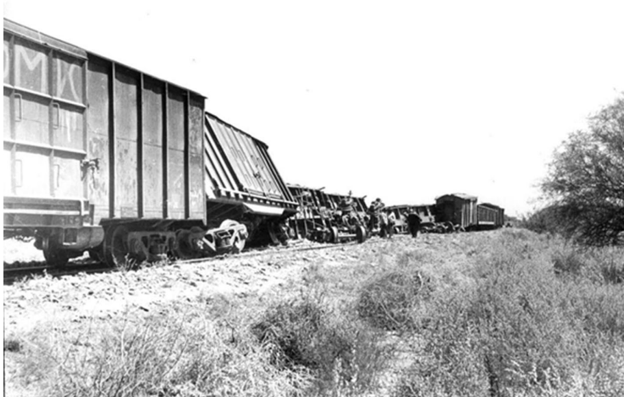
Fig. 3 Derailment of a freight train at approximately 31.5°S and 67.6°W that was traveling at a low speed due to the strong motion of the ( M_w 7.5) San Juan earthquake on 23 November 1977 (Photograph courtesy of the Instituto de Investigaciones Antisísmicas—UNSJ 1977)
