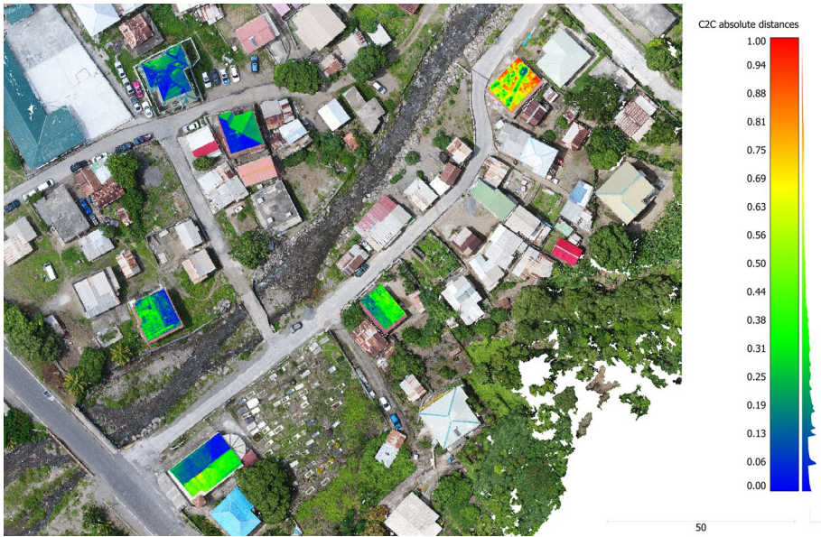
Fig. 6 Results from the alignment process using CC showing alignment error (CloudCompare, does not support TIFF output)
