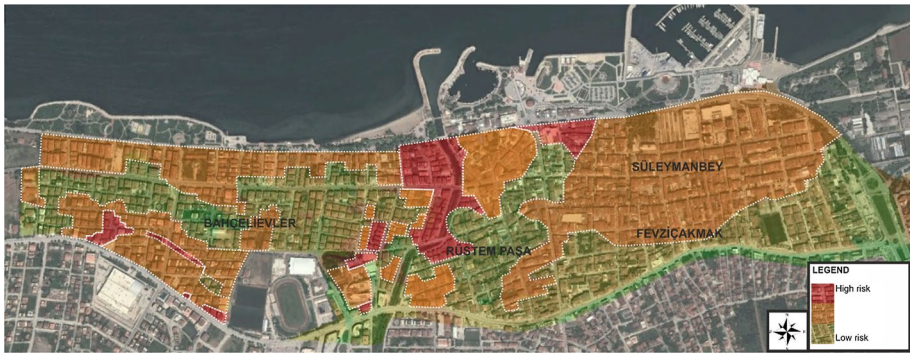
Fig. 3 AHP-1 map including geological criteria. The white dotted lines indicate the high and moderate risks. Therefore, areas having lower risk are separated from the high and the moderate ones
