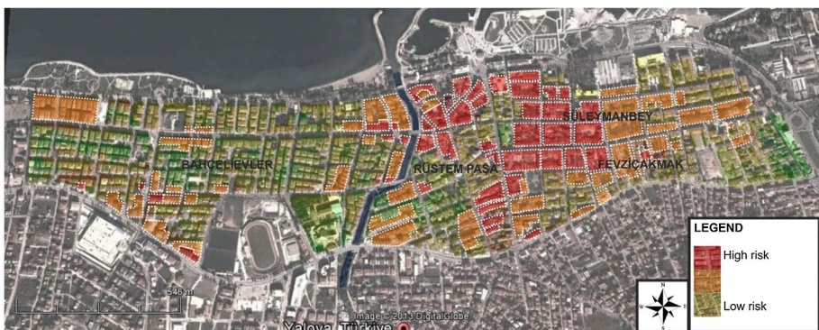
Fig. 6 TOPSIS map including both geological and superstructure/infrastructure criteria
