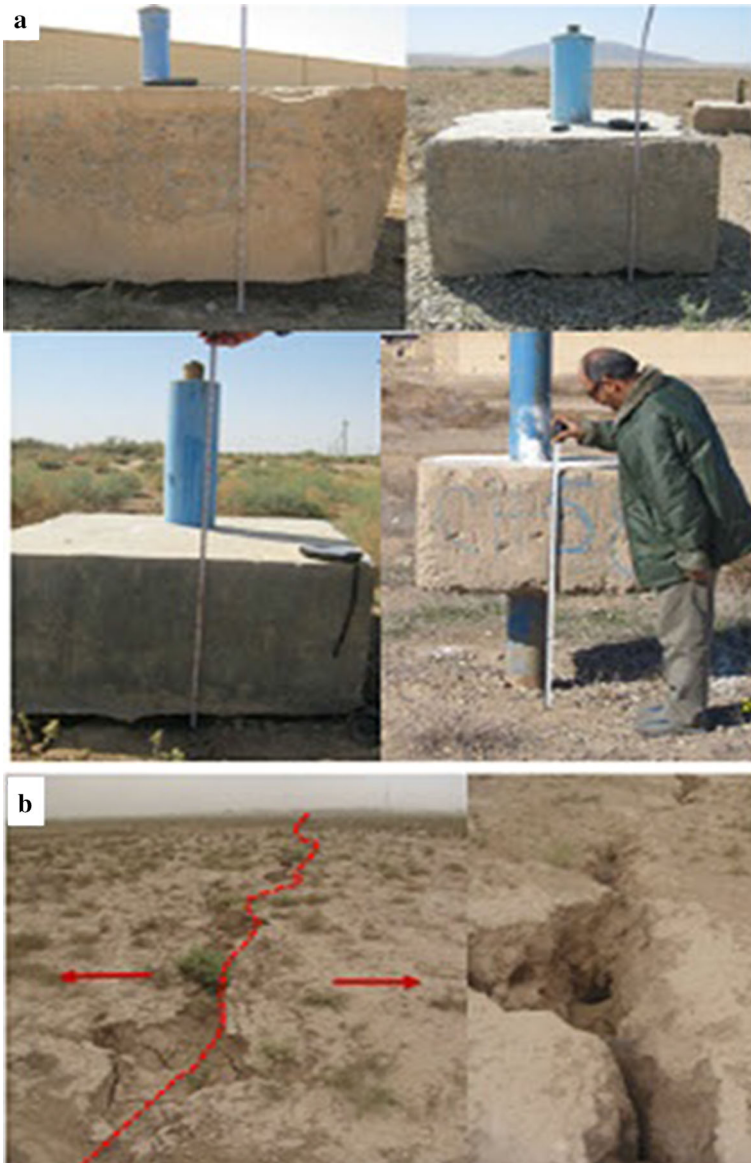
Fig. 1 a Subsidence in the vicinity of piezometers, b openings caused by subsidence near the Aliabad plain (Reproduced with permission from Qom Regional Water Company 2011a, b)
