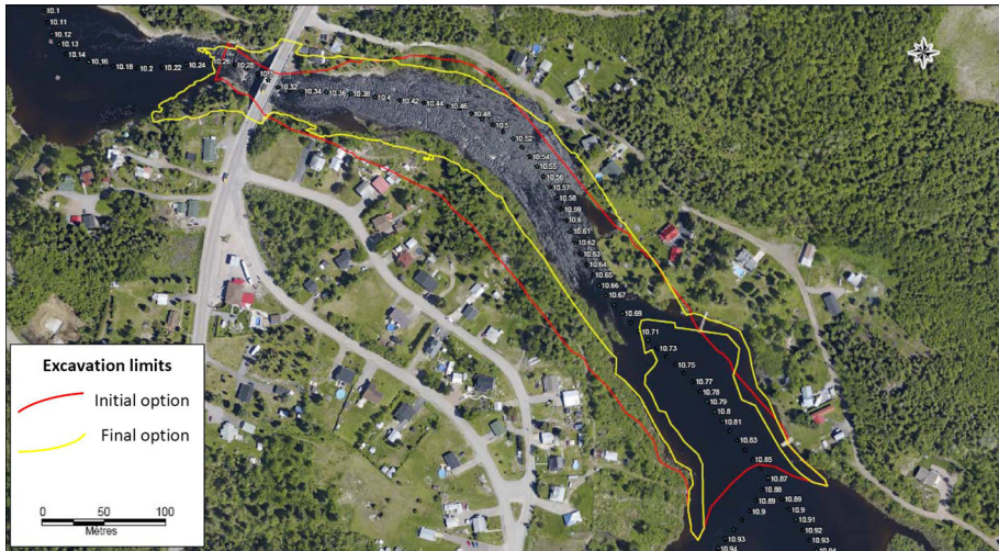
Fig. 6 Excavation limits from the Pibrac Bridge: yellow limits correspond to option replacing the bridge with a longer one with no pillar. (Modified after GENIVAR 2009)
