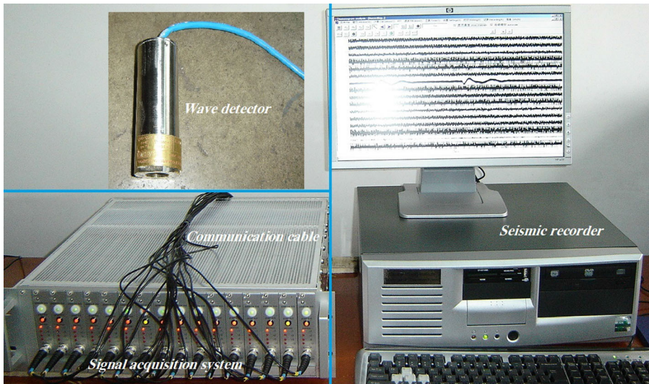
Fig. 6 Main components of the measuring instrument for the continuous microseismic observation
