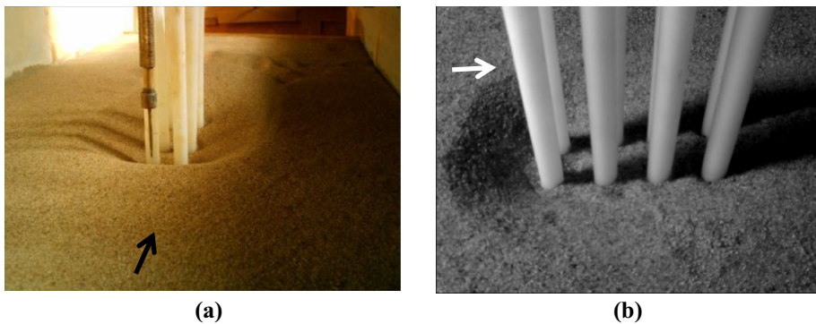
Fig. 2 Scour hole shape around PGs after the end of the experiments and dewatering the flume with arrows showing flow direction for experiments of: a Baratian (2007) and b Hajzaman (2008)
