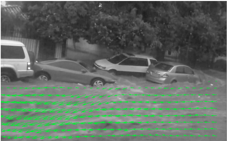
Fig. 4 Mean unrectified surface water velocity field obtained after implementing LSPIV technique. Arrows represent surface water velocity vectors
