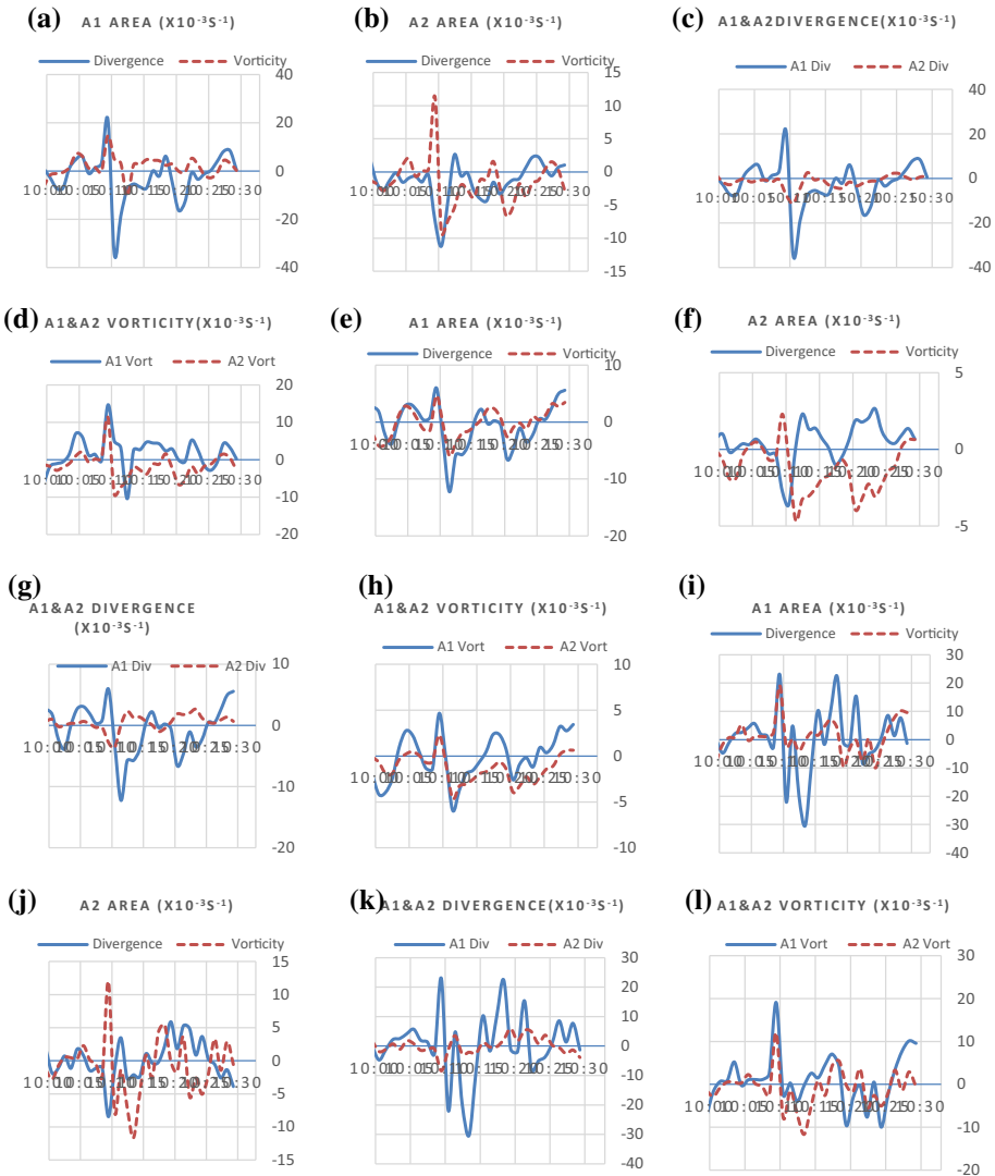
Fig. 18 Comparison of average divergence ( \times 10^{-3} \text{ s}^{-1} ) and average vorticity values that belong to A1 area and A2 area of Atatürk Airport on April 18, 2012, 1000 UTC–1030 UTC obtained by using maximum wind speed in 2-min interval; a A1 area, b A2 area, c divergence and d vorticity, by using average wind speed in 2-min interval; e A1 area, f A2 area, g divergence and h vorticity, by using instantaneous wind speed in 2-min interval; i A1 area, j A2 area, k divergence and l vorticity
