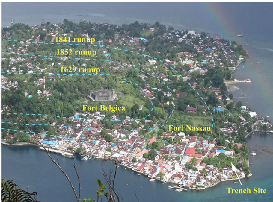
Fig. 6 Photograph of Banda Neira from the top of Banda Api (looking east). The inundation levels of three historical tsunamis that have struck to the island, including the 1852 event, are shown. The 1629 event is reconstructed by Liu and Harris (2013). The trench site location for Fig. 10 is shown
