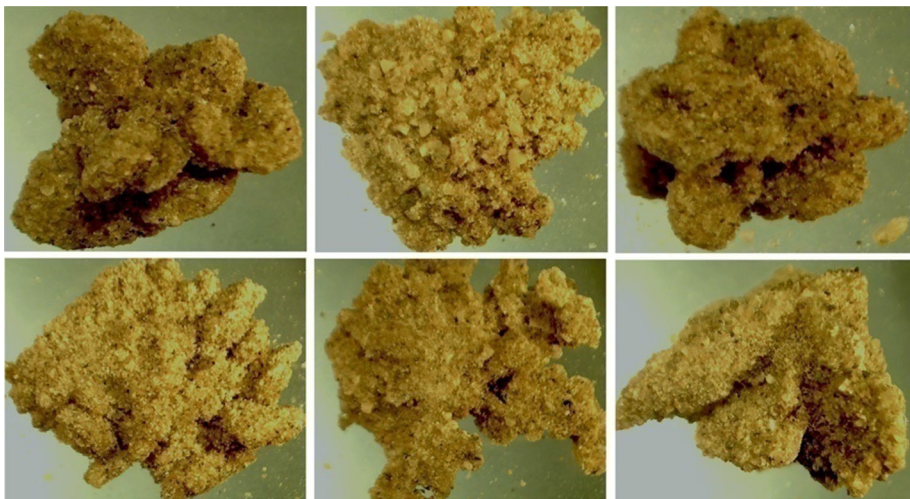
Fig. 2 The shapes of the SCB under the stereomicroscope (magnification: \times 50 )
