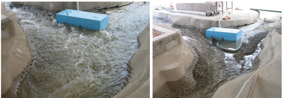
Fig. 15 Experimental photograph of sediment deposition near the hydropower plant
