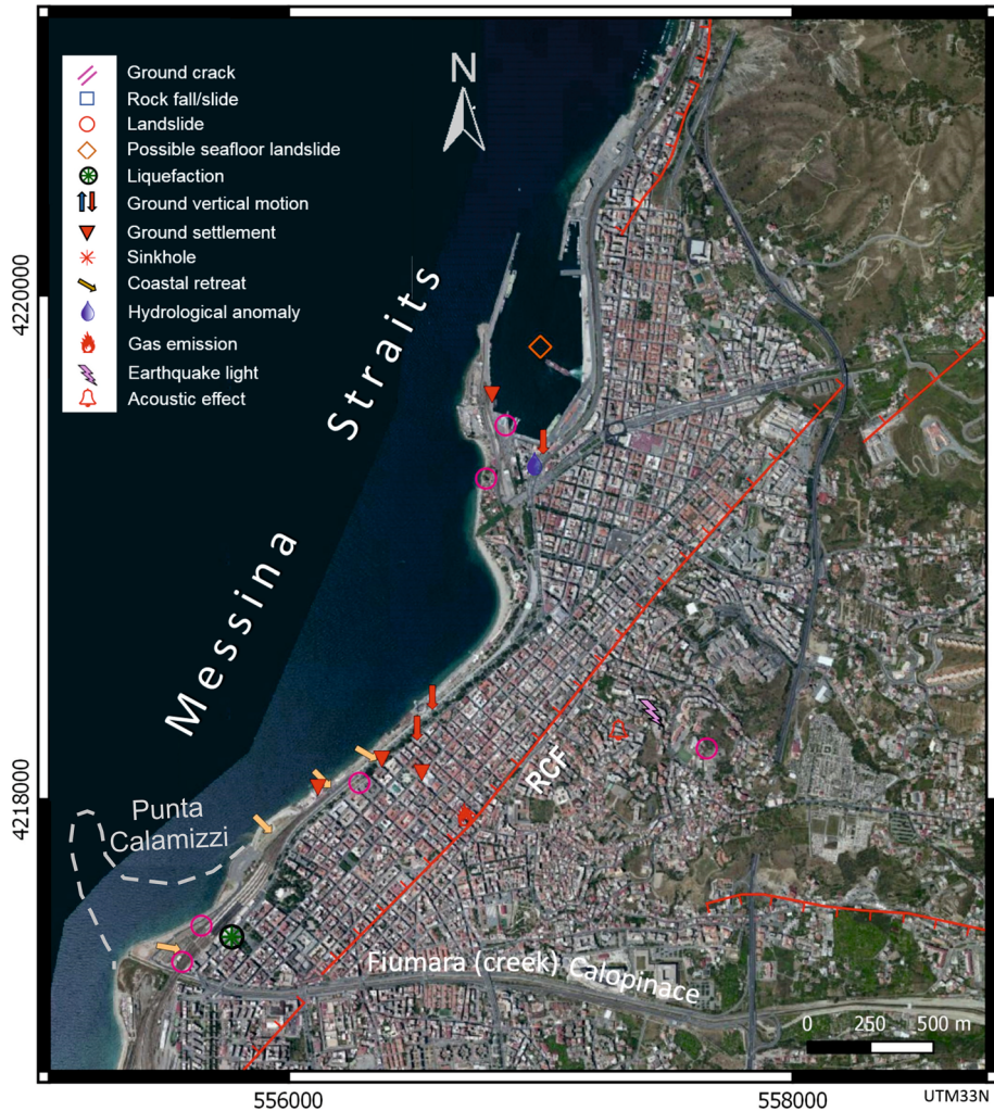
Fig. 9 EEEs occurred in Reggio Calabria. Most of these EEEs (erosion, subsidence, landslides, collapses) were reported along the seacoast. Faults from Atzori et al. (1983). The inferred shape of the Punta (Cape) Calamizzi that disappeared in 1562, likely because of a landslide induced by coastal erosion, is shown
