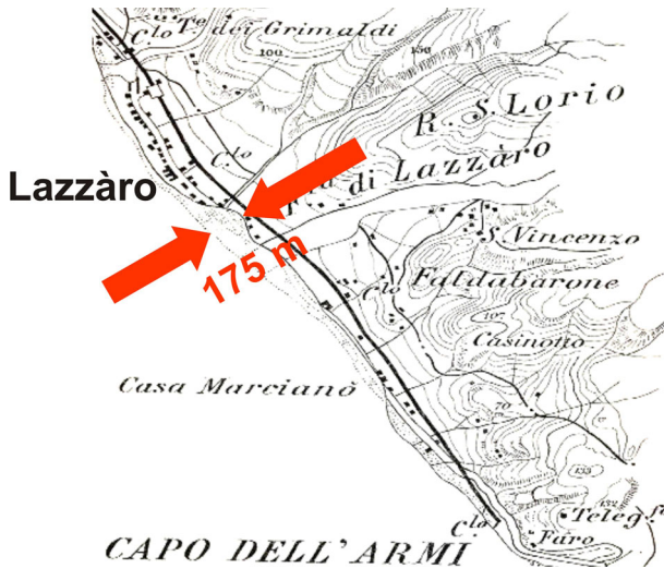
Fig. 12 At Lazzaro, the coastline retreated up to 175 m as a result of the cumulated effects of subsidence, earthquake shaking, and tsunami waves. After Novarese (1909), modified
