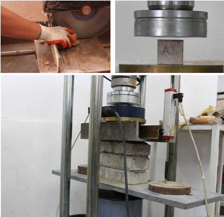
Fig. 6 The studies to determine the mechanical properties of the minaret stone
