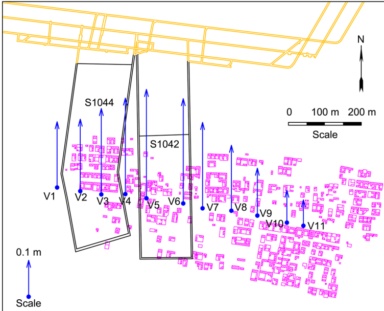
Fig. 11 Vertical displacement vectors of surface stations in the S104 mining section
