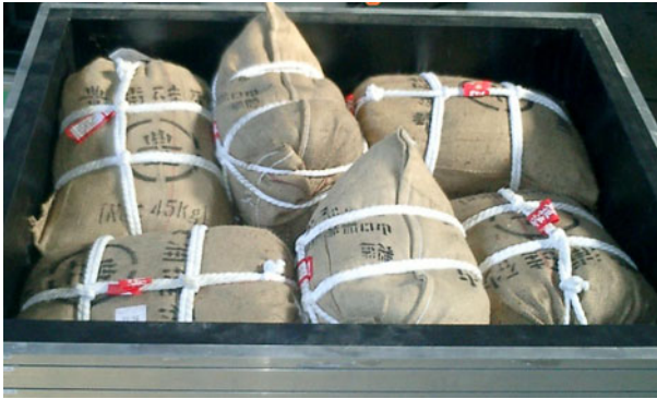
Fig. 11 Load applications in the laminar box
