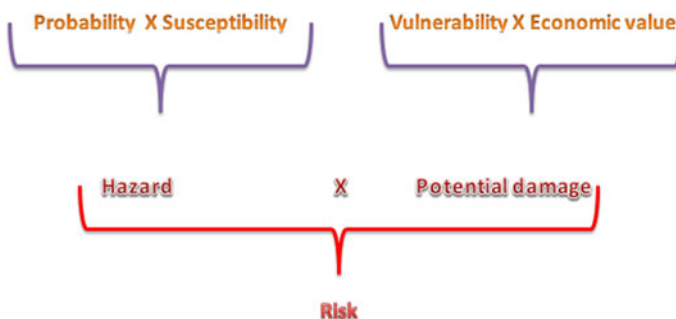
Fig. 1 Conceptual model of risk (Probability: fire occurrence probability in a position; Susceptibility: potential damage from the fire in a position; Vulnerability: degree of loss of a component at risk; Economic value: value (in €, $) of a component at risk) (MiSRaR 2010)
