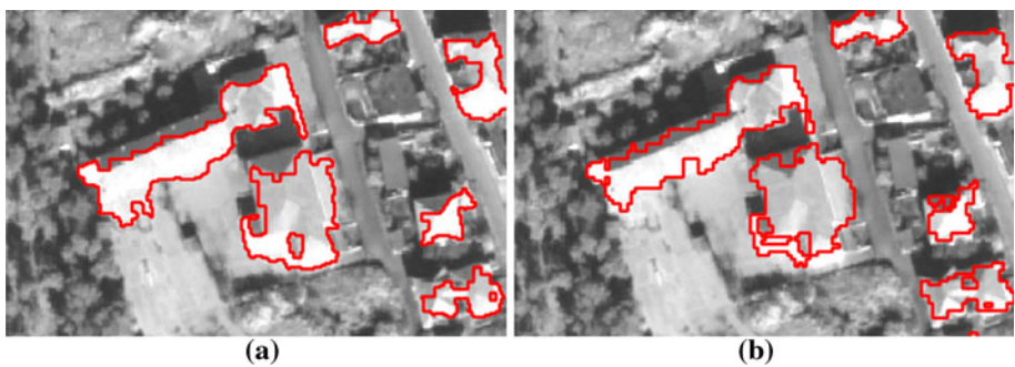
Fig. 6 Red lines define polygons with the outline of extracted buildings: a extraction using the unsupervised classification; b extraction using the supervised classification
