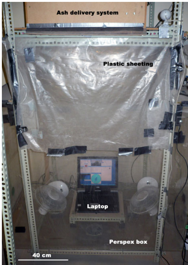
Fig. 1 The ash vulnerability testing chamber in test configuration with laptop and ash circulation fans inside. The ash delivery system and hopper injected ash into the chamber at a known rate. Plastic sheeting was used to contain the ash
