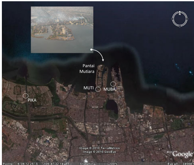
Fig. 12 Part of coastal areas of Jakarta, courtesy of Google Earth. In this figure, MUBA, MUTI, and PIKA are GPS stations with relatively large subsidence rates
