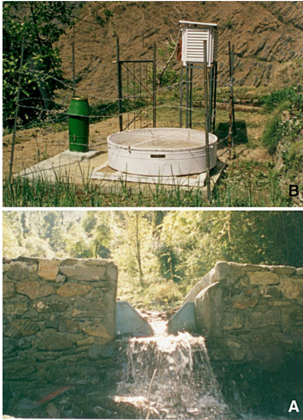
Fig. 4 a Hydrological station installed at the mouth of each sample micro-watershed. b Meteorological station installed at high altitude of each sample micro-watershed
