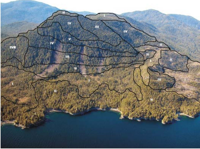
Fig. 6 Example polygons of five class terrain stability mapping. Projection is onto a landscape on the BC north coast. Classification is presented in Table 3
