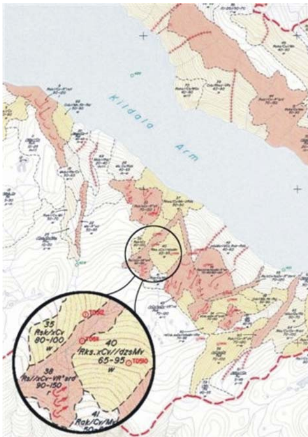
Fig. 4 Terrain map showing the terrain polygon number, terrain symbol, slope gradient, soil drainage, onsite landslide symbols, and the field inspection plots
