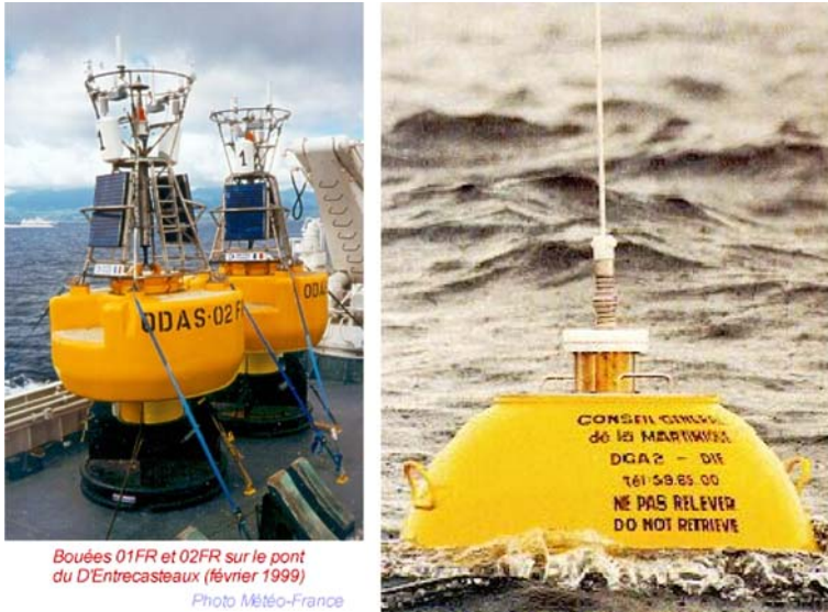
Fig. 2 The two MAWS buoys on the way for mooring ( left panel ), a directional wave buoy located close to Martinique ( right Panel )
