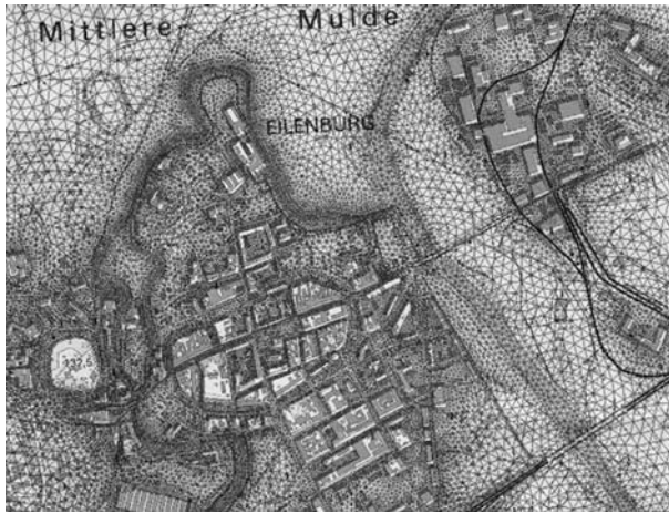
Fig. 6 Layout of the mesh of the full 2D-finite element model
