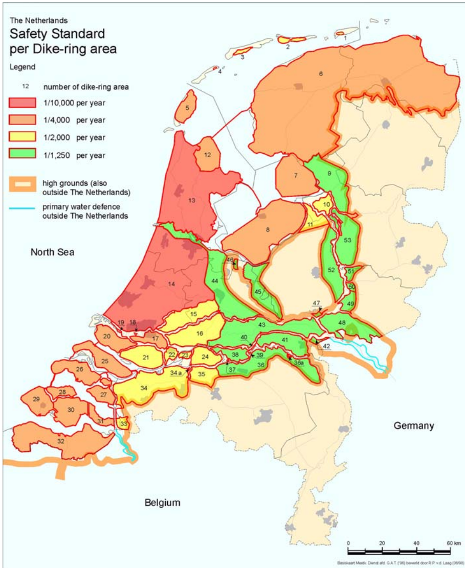
Fig. 3 Safety standards of Dutch flood defense system. In the densely populated western part of the country, the design return period is highest, T = 10,000 years. In the other parts of the country, the design return period is lower, T = 4000 years, T = 2,500 years, and T = 1,250 . From these design standards, water levels have been derived that have been used to determine the height of the dikes (Source: Ministerie van Verkeer en Waterstaat 2005)
