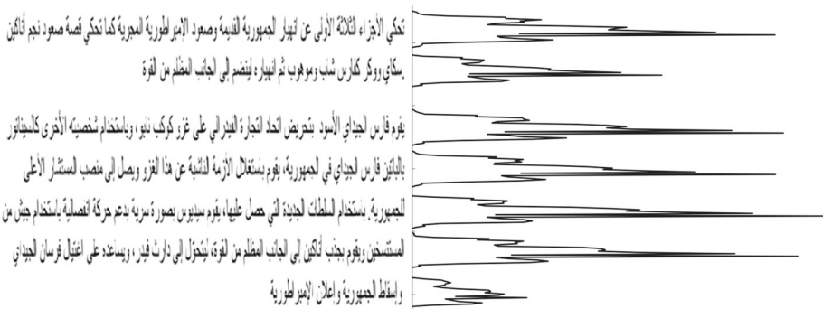
Fig. 4 Vertical histogram projection of Arabic text lines
