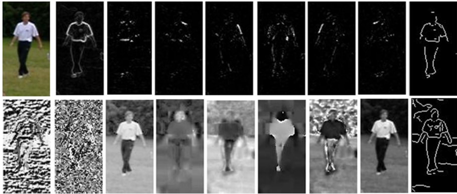
Fig. 1 Different channels of the input image (the first row gives the original, magnitude, gradient angle discrete from 1 to 6, sobel image, while the second row illustrates the lbp, orientation, luv, hsv and canny image)
