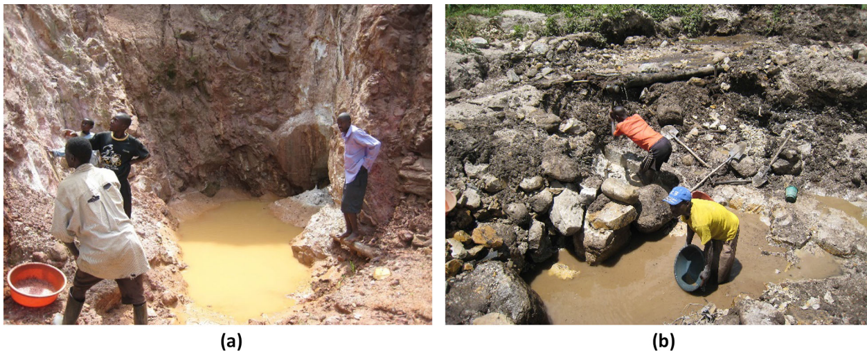
Figure 5. Artisanal gold miners working in the gold mine areas of a Mashonga and b Muti. At Mashonga, gold is in a steep NE–SW-trending shear zone composed of soft schistose material and kaolinized granite veins with only minor quartz veins. The soft mica-rich rock in the shear zone has resulted from strong deformation, hydrothermal alteration, and weathering into clay-rich material (Lehto et al., 2014b). The panning sites are located downstream from an old gold reef composed of a quartz stockwork in a light-colored sericite quartzite (or sandstone) matrix at Muti River workings. The river cuts this reef, which is most likely the gold source.
