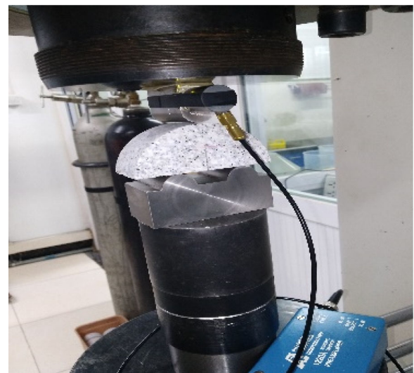
Figure 6. Semicircular bending test via the TAW-2000 series triaxial apparatus.
