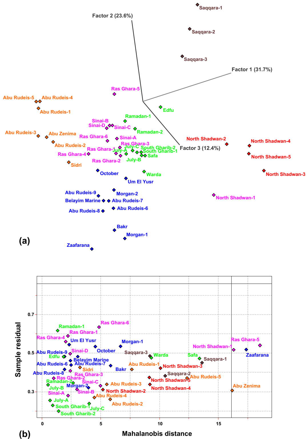
Fig. 18. (a) 3D view of principal component analysis (PCA) identifies oil families in the Gulf of Suez basin and (b) outlier diagnostics plot based on sample residual and Mahalanobis distance to emphasize confidence in the oil classifications. The oil samples are color-coded by family.
