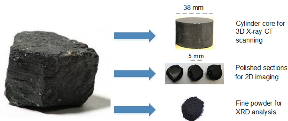
Figure 1. Sampling strategy for ScCO 2 -water saturation experiments and micro-structural characterization.
