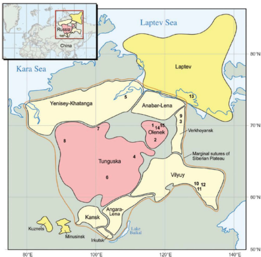
Figure 42. Eastern Siberia. Map of the sedimentary basins of the Siberian platform, Russia. Main heavy oil and bitumen deposit locations: (1) Olenek; (2) East Anabar; (3) Chekurovka; (4) Siligir-Markha; (5) Rassokha; (6) Chun'ya; (7) Medvezh'ye; (8) Turukhan; (9) Bulkur; (10) Tuolba; (11) Amga; (12) Sina; (13) Ust-Lena; (14) Kuoyka; and (15) Sololisk. Dark pink, uplift areas; yellow, basins (from Kashirtsev and Hein 2013).
